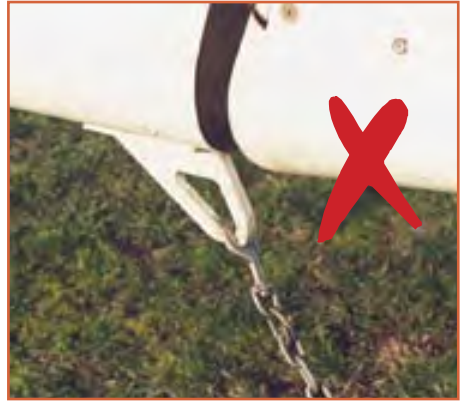
Dog-chain type clips should not be used when picketing, as they are not strong enough.
