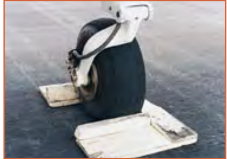
Chock the main wheels fore and aft.
