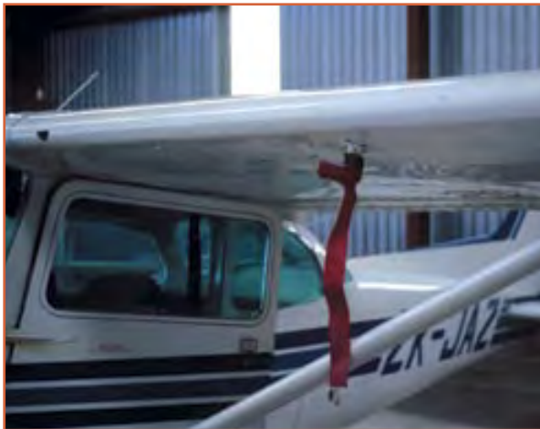
Pitot tubes should be covered to prevent the ingress of windblown dust and dirt. Remember to remove the cover before flight!
