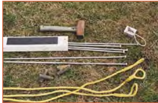
A lightweight set of pickets utilising stainless steel rods and twisted shackles stored in a plastic (downpipe) tube.
