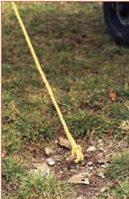
Check the type and condition of your tiedown rope. Nylon or dacron rope is recommended.
