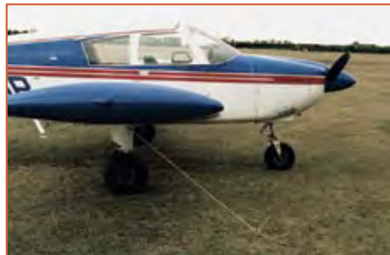
The underwing ropes should be led to points outboard and forward of the underwing attachment point. Pickets should be hammered into the ground in front of the wing.
