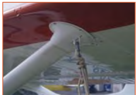
Tiedown ropes should only be tied to the aircraft tiedown rings.
